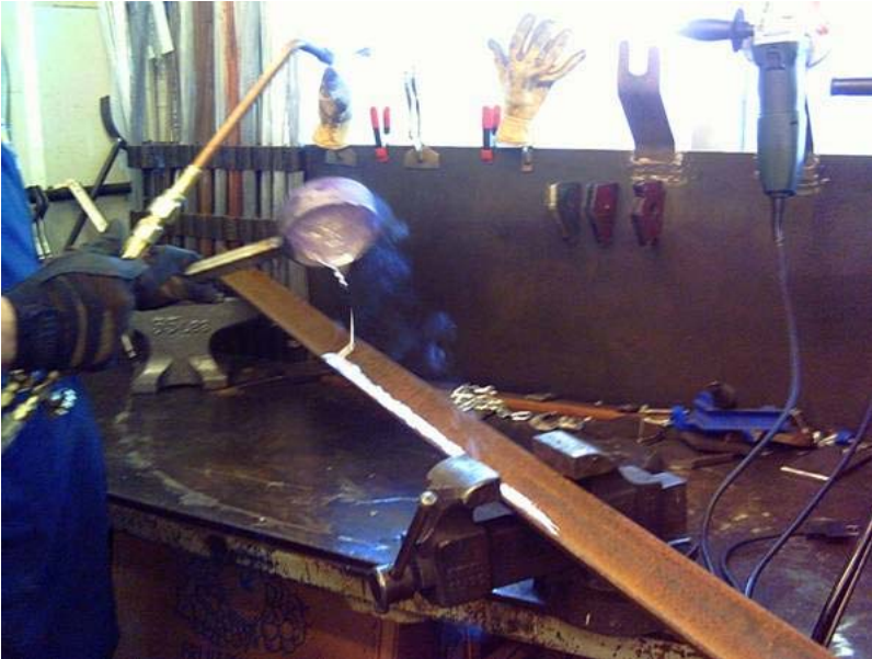
Molten aluminum poured onto rusted steel: no violent reactions observed at all.
