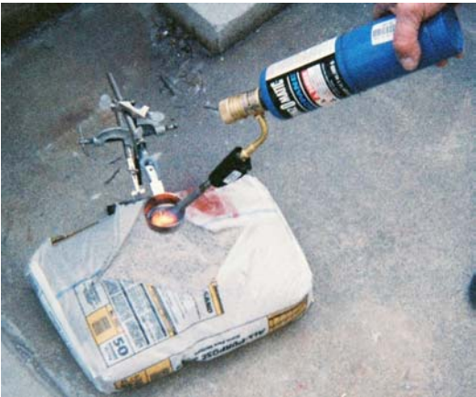
Thermite did not ignite when heated with a propane torch.
