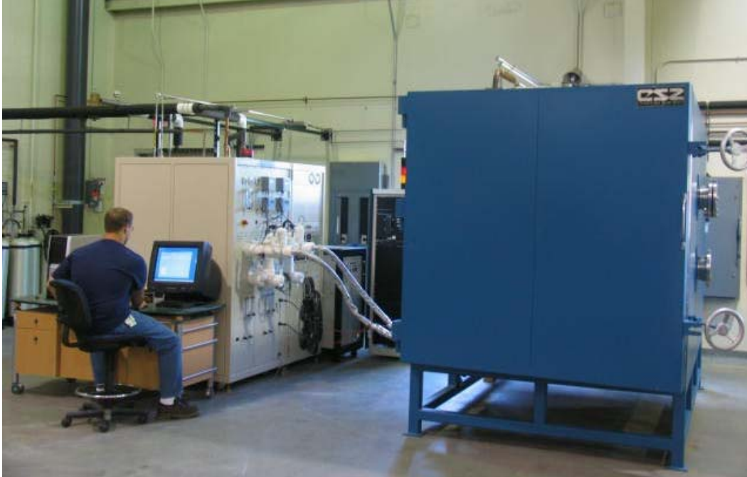
NSWC-Crane Fuel Cell Test Stand Integrated with Altitude Chamber
