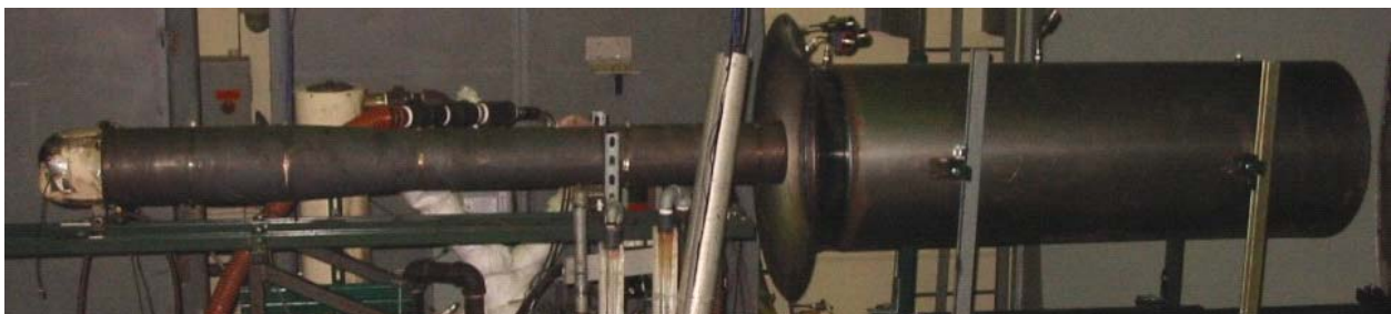
Pulsejet-Driven Ejector installed on the Pulsed Detonation Research Facility's damped thrust stand
