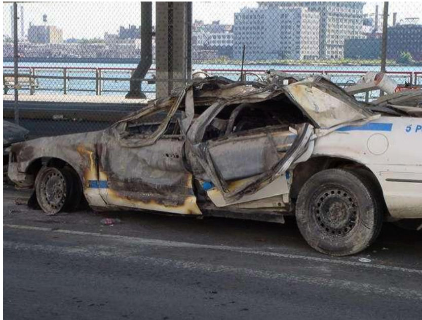
Figure 39. Peculiar wilting of car doors and deformed window surrounds on FDR Drive.
