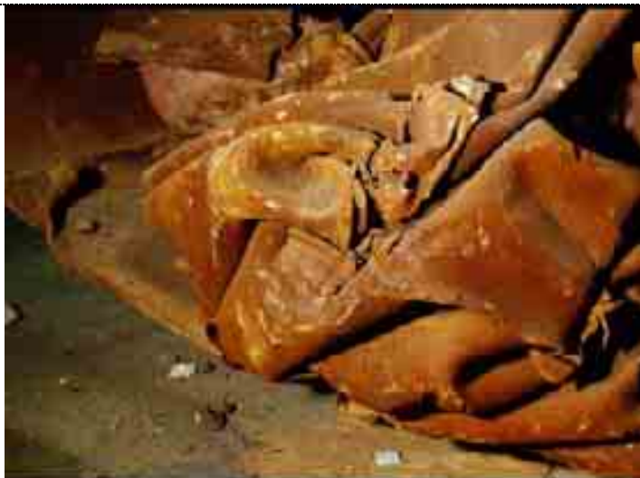
Figure F-A-2c: Collapsed part of Column 210.
