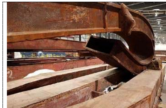
Figure 115. WTC core column curled, not buckled. A gravity-driven "collapse" would not do this. The beam above has smooth curves, without kinks. (2002)
