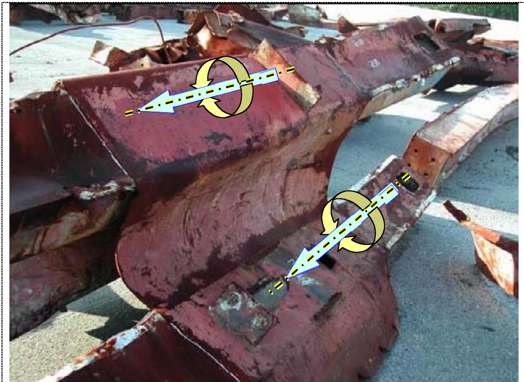
Figure 140. The spandrel belt looks like a wet tissue was draped across the beams and spraypainted bright red. Rigid once again.
