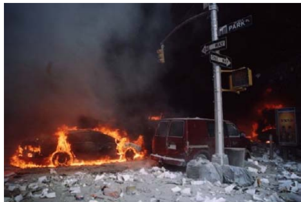
Figure 51. The tires and even the pavement under the car are on fire. The windows appear to be intact with no visible interior fire. There is line of fire along the trunk lid. The right front fender is deformed and has turned white.
